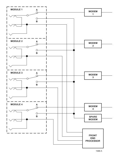
Figure 1-1. Typical Hot Spare Modem Configuration
